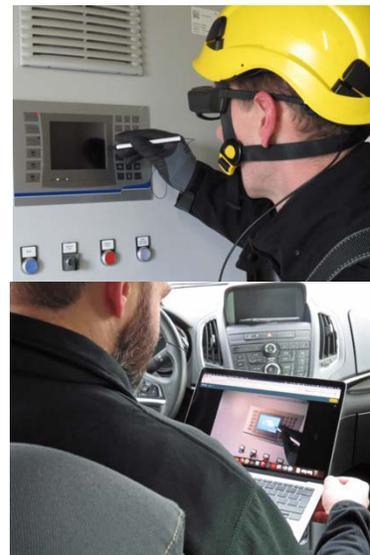
*Figure 2: A Field Service Technician uses Iristick Smart Glasses to stream a live view to another technician for remote assistance.*
