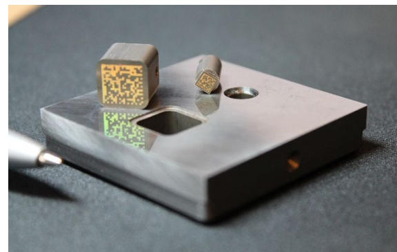
Rel8's imZERT™ technology arranges nanostructures to engrave DPM barcodes as small as 1mm 2 into molds.
